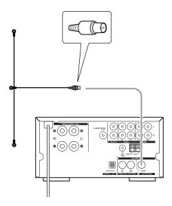
• You can check the antenna adjustment or positioning for the best reception by viewing the signal strength on the display.
